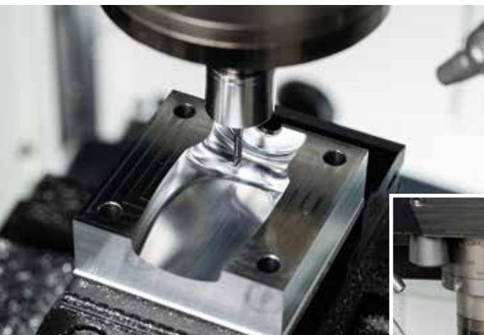
For semi-finishing, the team opted for a HORN ball-end mill having a diameter of 4 mm
