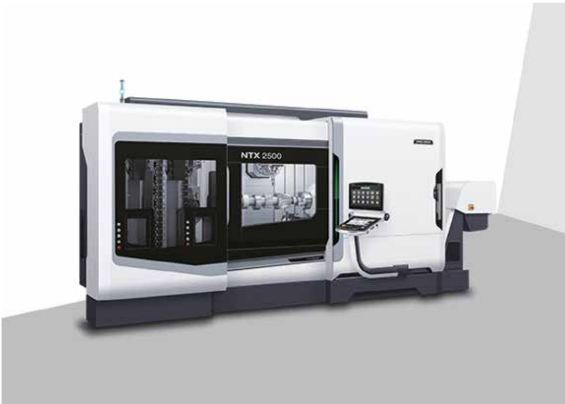
The NTX 2500 2. Generation from DMG MORI enables complete turn-mill machining of the titanium component. Turning, drilling, simultaneous 5-axis milling, and in-process measurement, along with AI-based CELOS X widgets and technology cycles, work together to ensure a manufacturing process that is both stable and highly precise (Pictures: DMG MORI)
