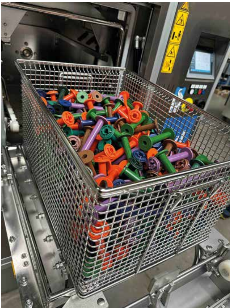
Cleaning and drying plastic parts in bulk in a washing basket (Pictures: BvL Oberflächen-technik GmbH)
