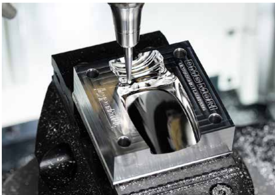
High-polish milling eliminates the need for polishing (Pictures: HORN/Sauermann)
