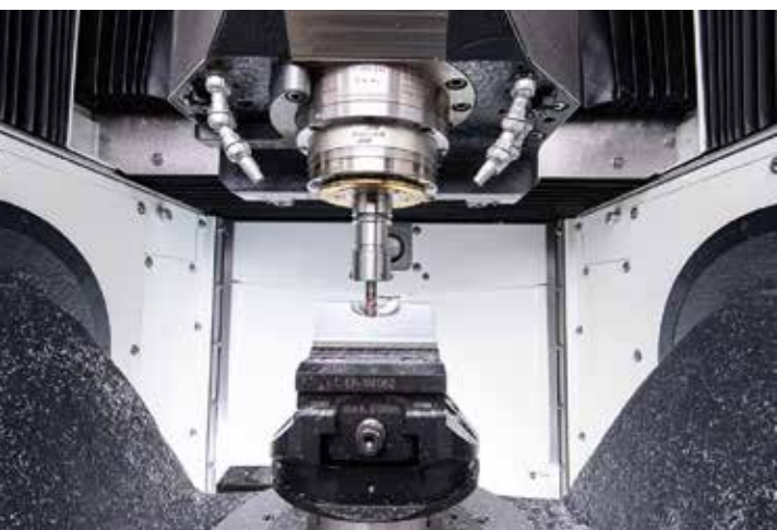
A 16 mm Horn end mill from the DS system was used for roughing
