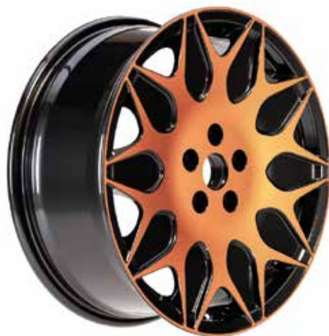
The new light-performance wheels are up to 20 percent lighter than conventional low-pressure die-cast wheels
