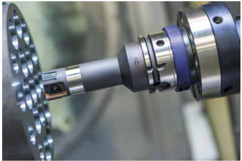
Chip breaker geometry for long-chipping materials: Precisely defined lead and rake angle geometry, combined with adapted cutting data and depths, enables perfect chip formation for long-chipping steel materials (Pictures: ©MAPAL)
