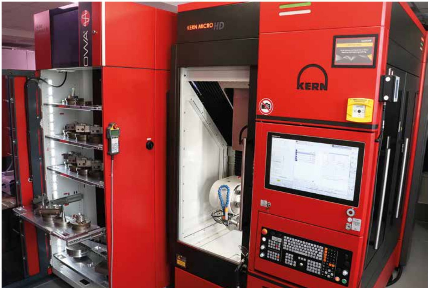
In use at toolcraft since 2024: the Kern Micro HD five-axis precision machining center equipped with a grinding package
