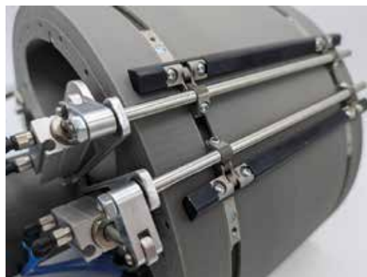
Stainless steel clamping set mounted on a model of the imaging drum of the XStream thermal plate-setter by Krause Biagosch. The XStream is used for imaging printing plates in the graphic arts industry (Picture: © Krause DiMaTec GmbH)
