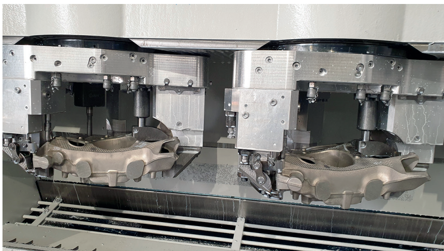
Production at Schabmüller mainly takes place on multi-spindle machines. Hub carriers are machined by SW on a double spindle
